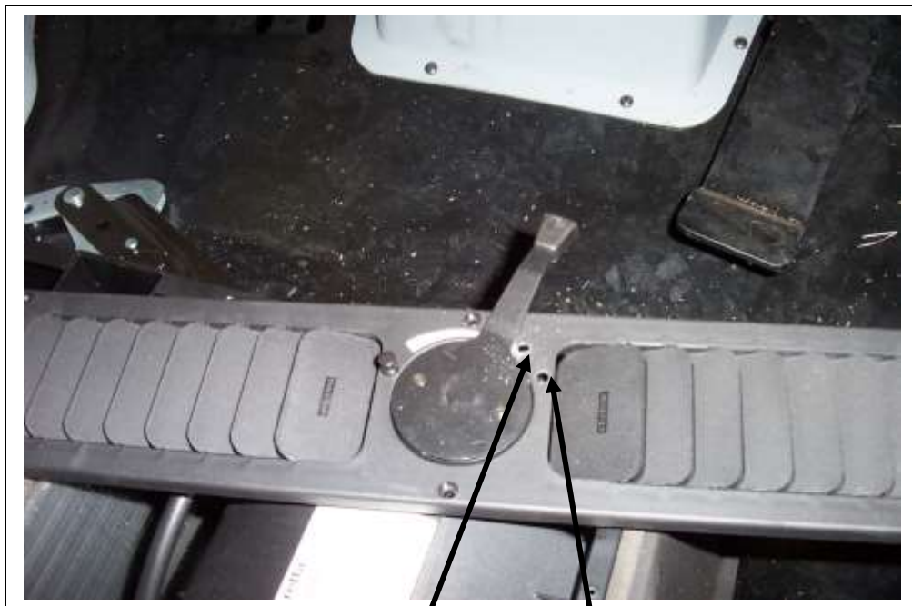
New stop location for inside air control handle. Drill a new hole the same size as the original hole.
