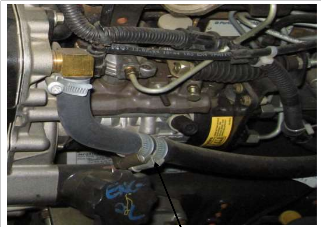
Clamp off heater lines on both sides of splice
