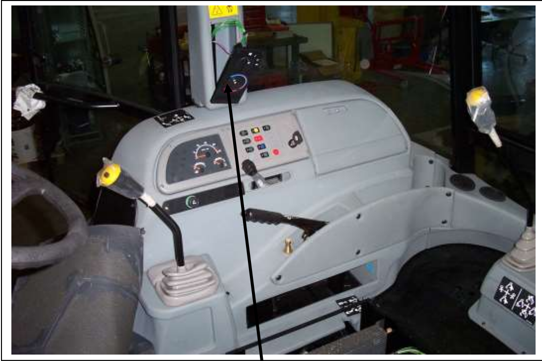
Heat/AC control panel unscrewed from frame
