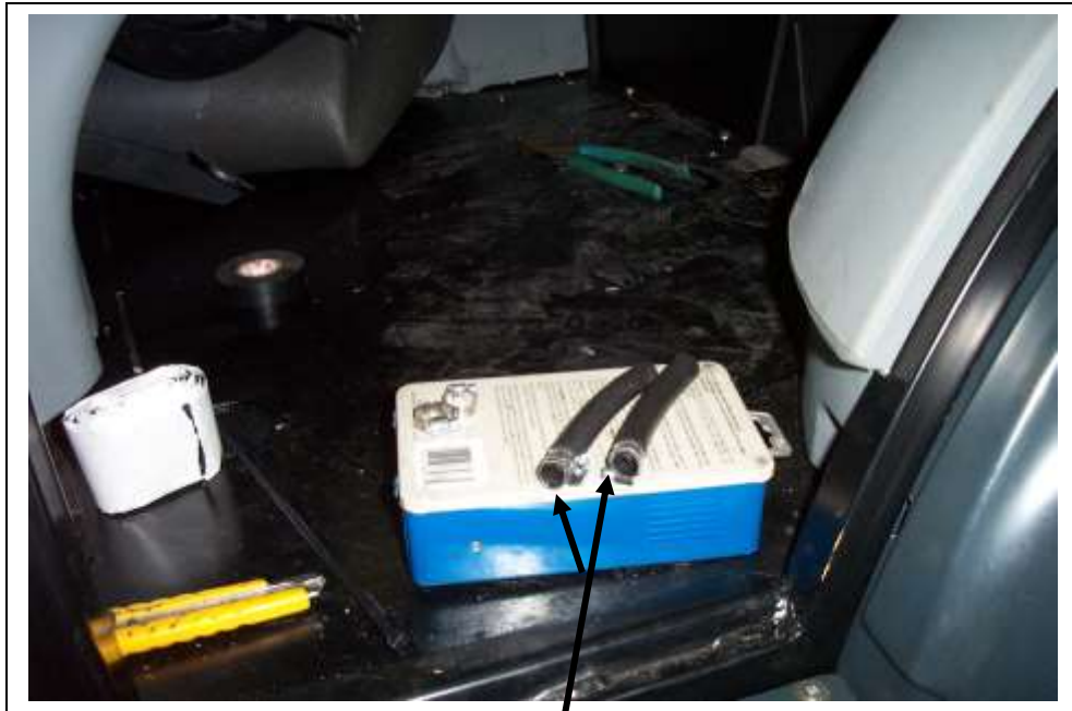
Drain tubes with restrictors installed ready to attach to the drain tube extensions
