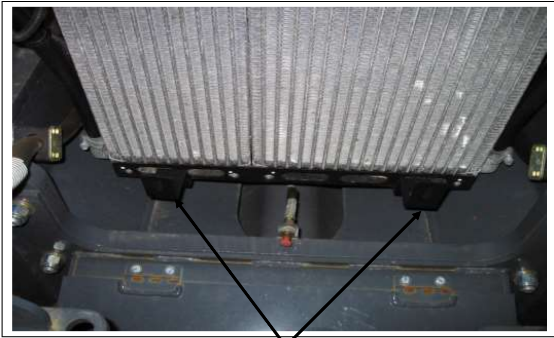
Lower condenser mount brackets installed loosely.
